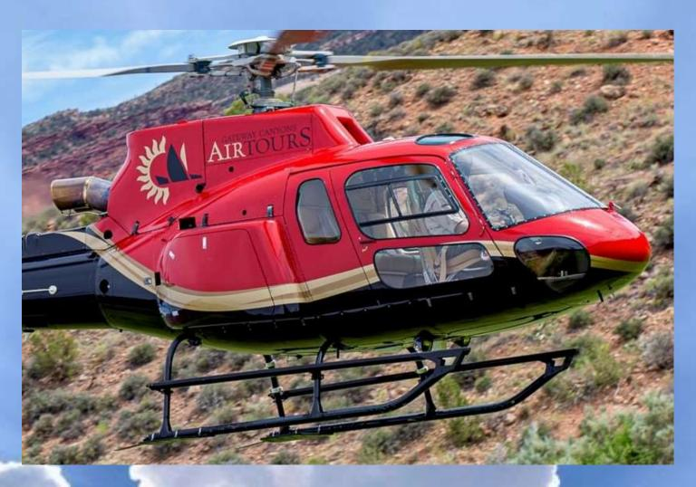
The helicopter is equipped with a highly reliable Turbomeca Arriel 2B1 engine. The AS350B-3 model is known worldwide for its superior reliability, and unmatched strong and safe performance at hot and high altitudes. Unquestionably the AS350B-3 is the industry leader for operations at high altitudes and hot temperatures.
