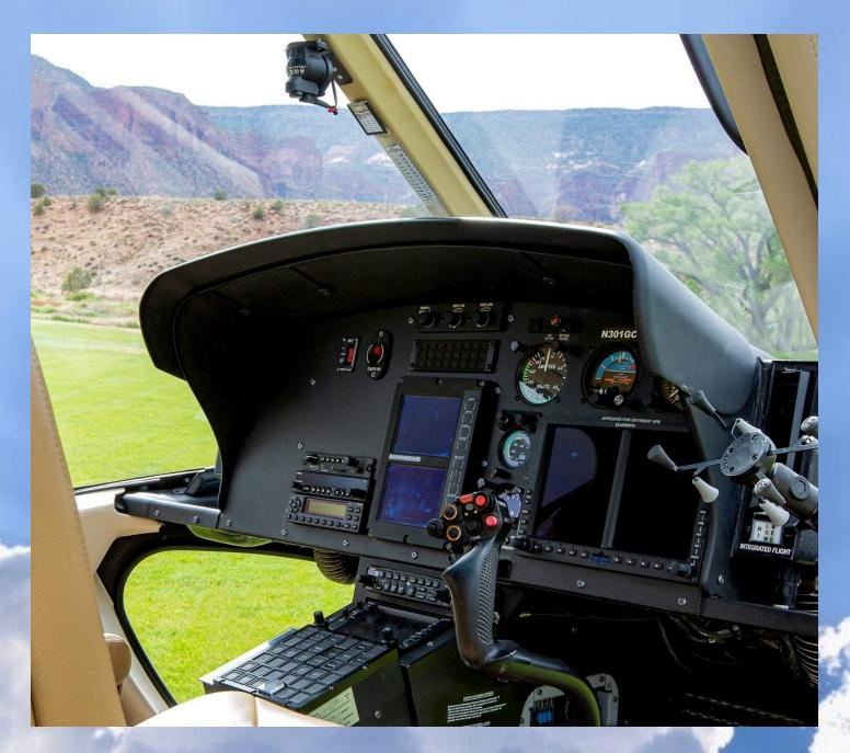
The avionics are certified for VFR operation, with VFR instrumentation. Additional avionics are installed qualify this AS350-B3 to be used for IFR instruction. Additional avionics are required for actual IFR flight. The Garmin avionics suite is equipped with ADS-B and includes a G-500H Dual EFIS display with synthetic vision and chartview accompanied by a GMA-347H audio panel, a GNS-430AW GPS/Nav/Comm with WAAS, a SL-30 Nav/Comm, a GTX-328 transponder and GDL-69 datalink.
