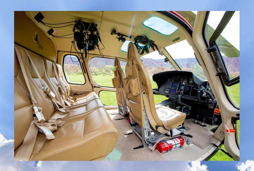
The executive interior of this AS350B-3 offers four seats in the aft cabin with each seat having its own noise cancelling headset interfaced to an intercom system for comfort and communication with your other guests. Up front the right seat controls are removable for a fifth passenger providing a total of five (5) passengers and a pilot. This executive helicopter is equipped with air conditioning for a "cool" comfortable ride on the hottest summer day.
