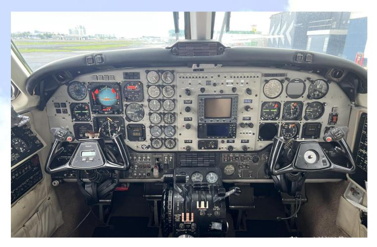
The Collins avionics suite includes dual nav radios, dual VHF transceivers, a DME, an ADF and dual transponders. Additionally the cockpit has been upgraded with a Garmin GPS-400 GPS/moving map, a Garmin transponder and ADS-B.
